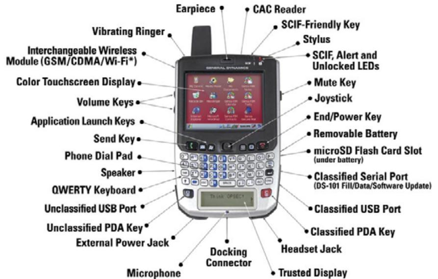
*The Sectera® Edge™ smartphone converges secure wireless voice and data by combining the functionality of a wireless phone and PDA — all in one easy-to-use handheld device. Developed for the National Security Agency's Secure Mobile Environment Portable Electronic Device (SME PED) program, the Sectera Edge is certified to protect wireless voice communications classified Top Secret and below as well as access e-mail and websites classified Secret and below.*
