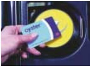
The scheme is operated by TranSys (a consortium of Cubic, EDS, Fujitsu and WS Atkins) and is based on Philips' Mifare standard 1k chips. Travellers wave the card over a distinctive yellow circular reader (a Cubic Tri-Reader) to 'touch in' and 'touch out' at the start and end of a journey. The Oyster Card was aimed at keeping London's public transport moving faster and more efficiently. According to figures from TfL, as of March 2006 over 5 million people now use the Oyster card.
