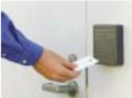
The two major contactless Smart Card standards today are International Organization for Standardisation (ISO) 15693 and 14443. Both standards define the protocols, data formats and other features necessary to ensure that contactless Smart Cards can communicate with readers and applications that adhere to the same standard. However, it's important to note that as far as reader-writer devices are concerned, supporting one standard does not lock out other options.
