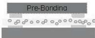
**FIGURE 2:** ACF film before assembly, with the spheres uniformly distributed and making no electrical conducting paths.
