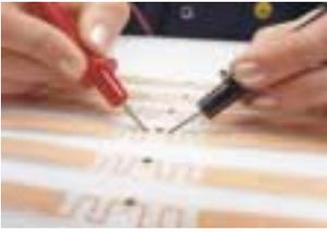
In order to make sure that production runs smoothly and outgoing quality is always good, we test each and every tag that leaves our factory. Monitoring includes both functional testing of the tag as well as the testing of important electrical characteristics. Not only can we adjust process parameters according to the outcome of the tests, but we also keep a log of the results so that we have full trace-back capability."
