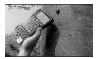
Radio Frequency tags are being used to identify and keep track of individual trees for safety, maintenance, conservation and woodland management.
