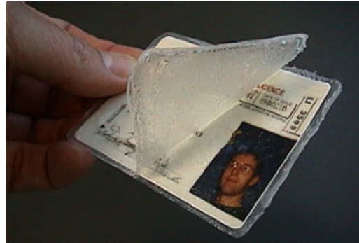
Figure 1: The photograph and personal details can be easily changed on laminated cards by separating the layers.
