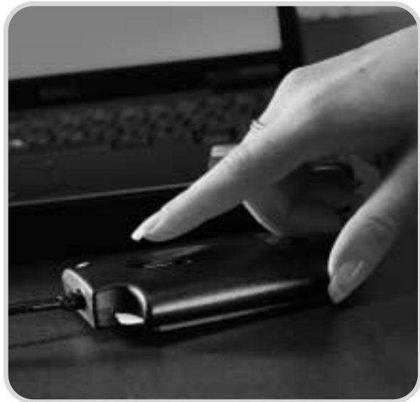
Fingerprint identification with Miotec's biometric PKI card and Precise Biometrics card reader
