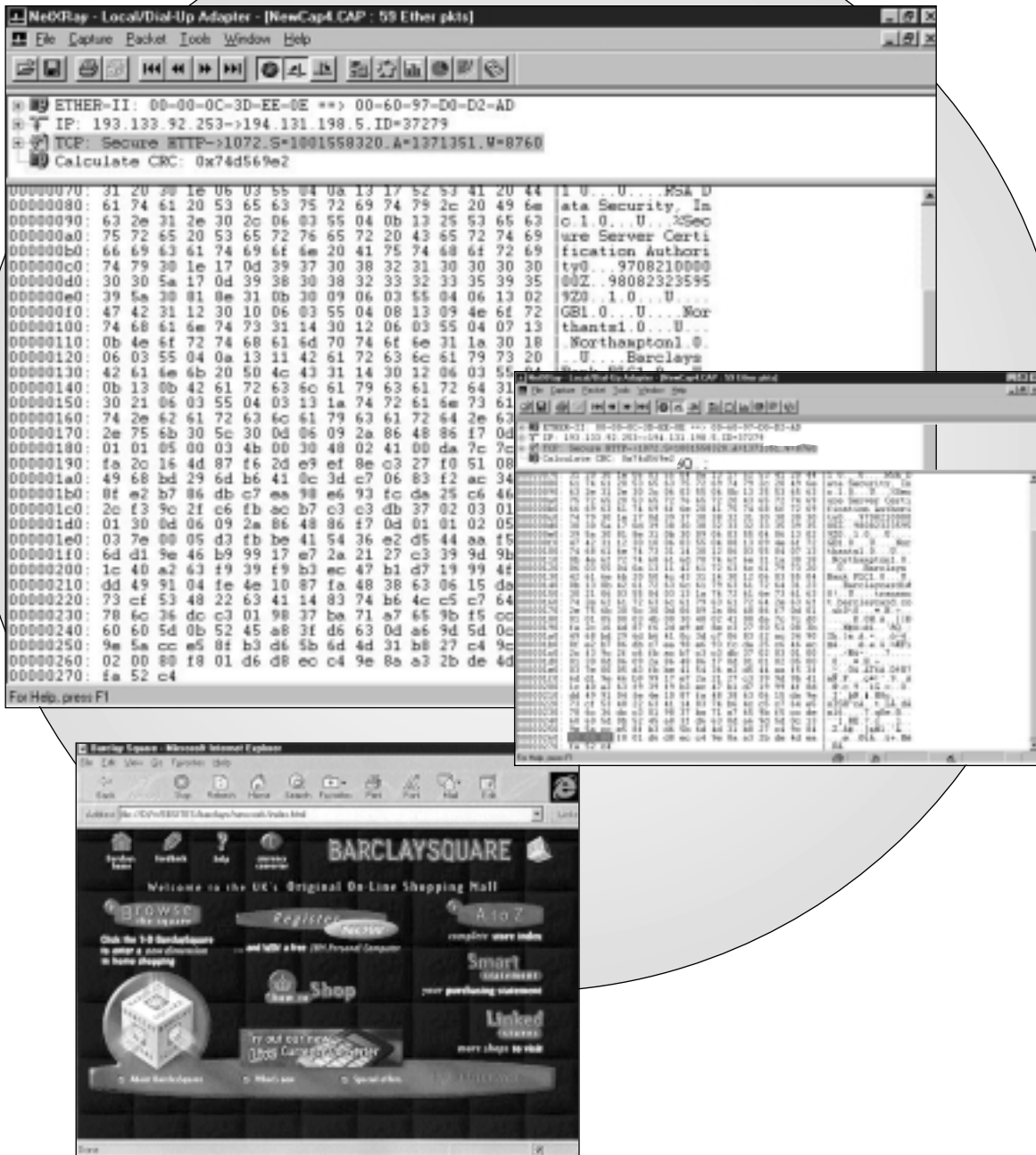
Right: Figure 4 SSL on Barclay Square The Server Hello response indicates that the server will use RC4_128_EXPORT_40_WITH_MD5 (see highlighted part in the second screen shot).
